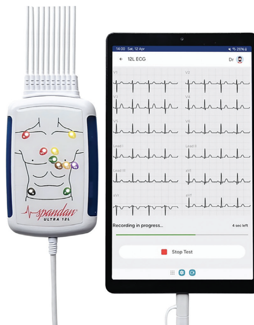
Figure 1. Integration of Spandan Ultra 12-lead ECG device with smartphone for data acquisition
